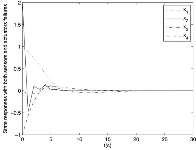
Fig. 4. State responses for NNCS with unreliable sensors and actuators with different failure rate.
