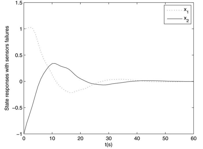
Fig. 2. State responses of the system with unreliable sensors having different failure rates.
